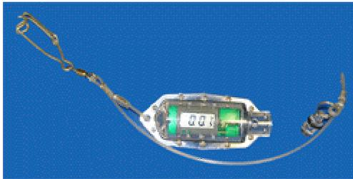
The HT 600 is a physical event timer suitable for underwater use. It was designed to acquire accurate data for bait take or time of interaction for longline fishing.
